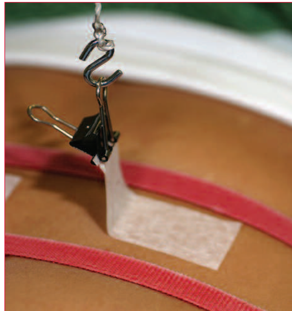
Figure 2: Use of thin straps to reduce deformation of the skin during the in vivo peel test.
